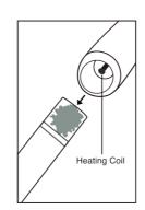
Flip over the Integrated Mouthpiece and Chamber. Load the ground herb into the Chamber
